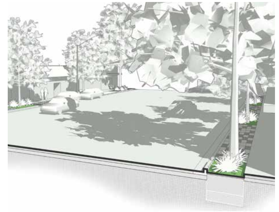
Figure 9-2. Tree Wells along a High-Volume and Speed Street.
