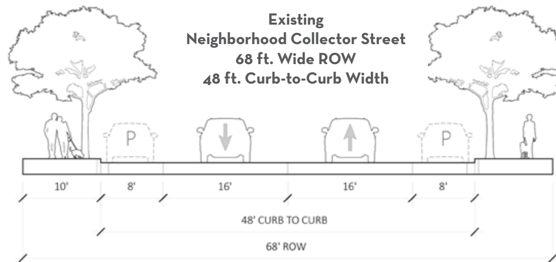
Figure 7-10. Existing: Typical Neighborhood Collector with a 68 ft. wide ROW and 48 ft. wide curb-to-curb.
