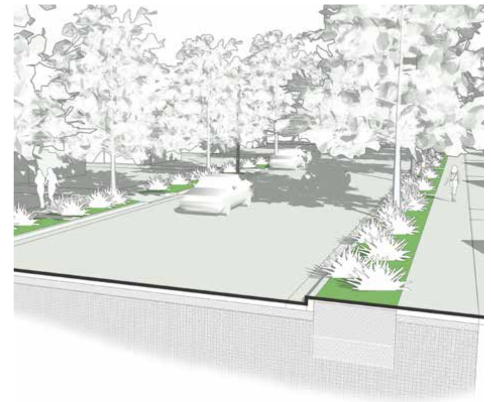
Figure 9-3. Planters along a Low-Volume and Speed Street.
