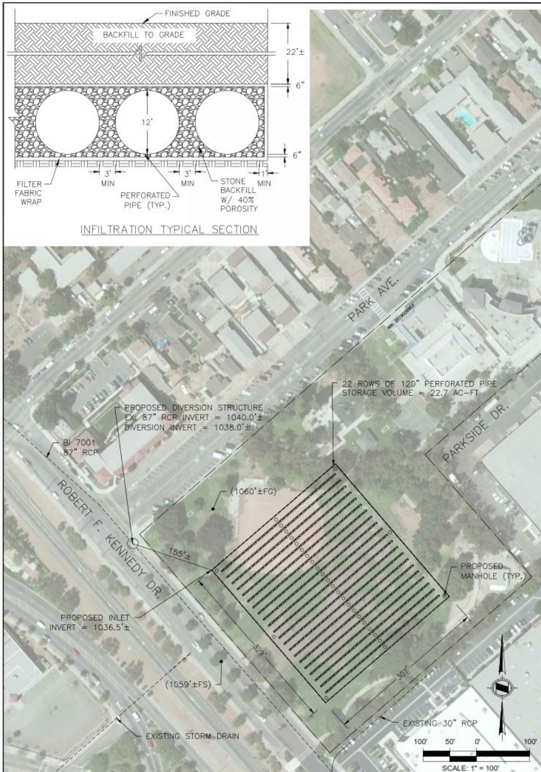
Figure 4-27. San Fernando Park Subsurface Infiltration Concept
