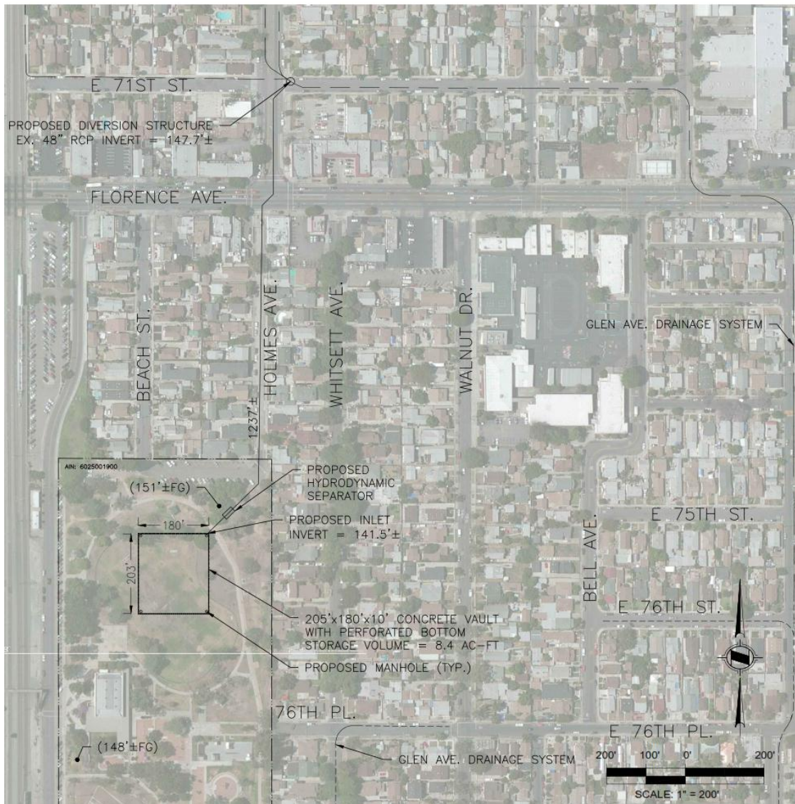
Figure 4-19. Roosevelt Park Subsurface Infiltration Concept
