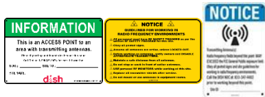
Post at all Sloped Roof Access Points
