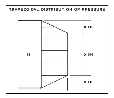
Shoring restrained by bracings or tiebacks and supporting a level backslope may be designed utilizing a trapezoidal distribution of pressure as indicated in the following table:
