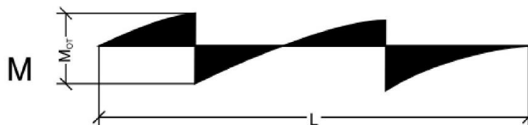
Figure 5-32 Moment distribution in the concrete grade beam.
