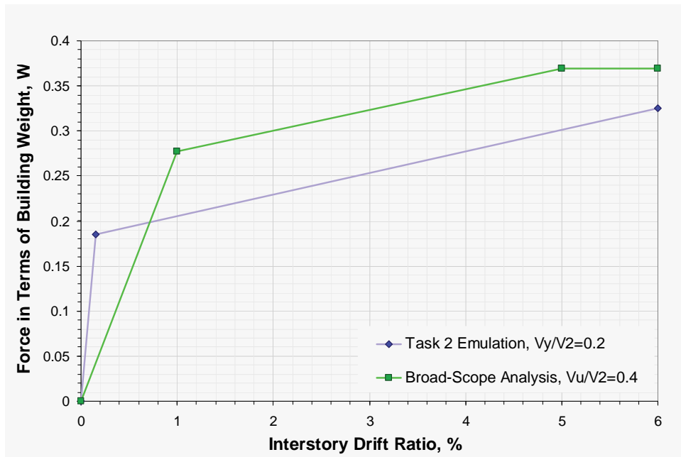
Figure F-12 Comparison of backbone curves for Task 2 retrofit set with ratio V_y/V_2 = 0.2 , and Broad-Scope Analysis retrofit set at V_u/V_2 = 0.4 .
